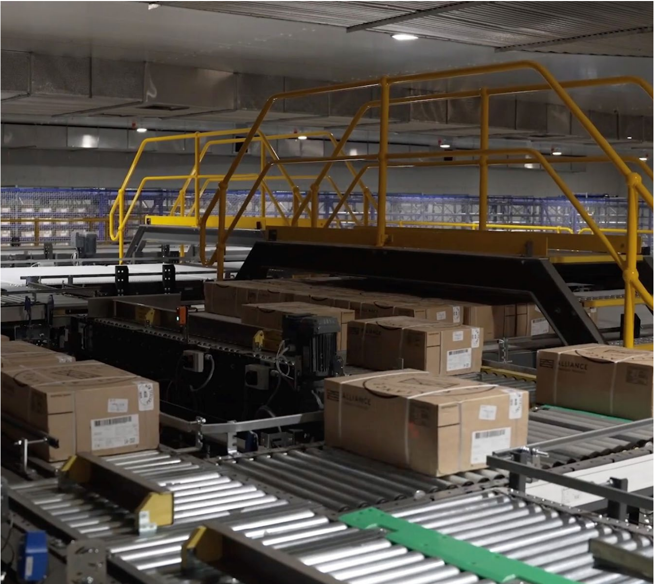
Product is automatically moved through the warehouse and palletised without being touched by human hands at our Lorneville plant near Invercargill.
