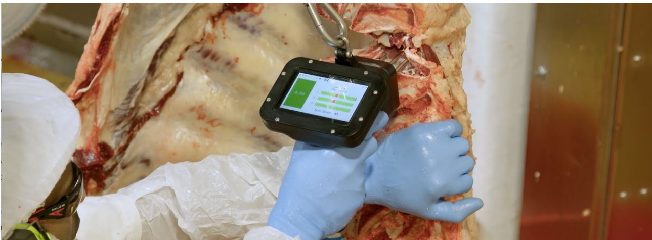
The MEQ probe – used to measure intramuscular fat (IMF) levels in lamb and marbling percentages in beef.
